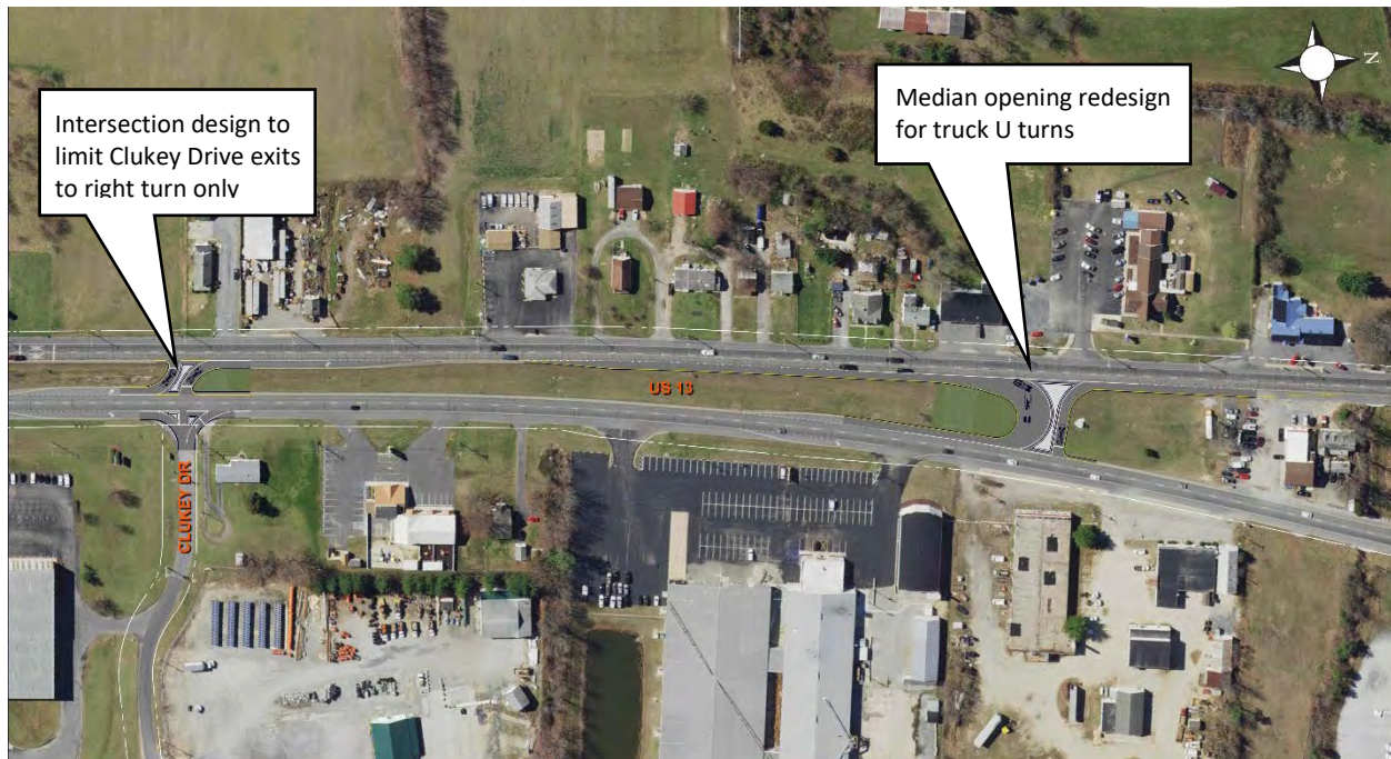
Figure 13: Clukey Drive Access Modifications
