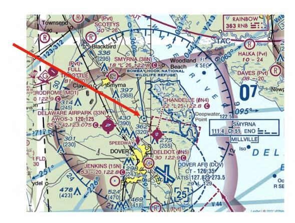
Figure 79: Smyrna VORTAC, represented by a hexagon symbol on VFR sectional charts. Note the frequency, TACAN channel, and Morse ID of the facility are also listed. Source: FAA.
