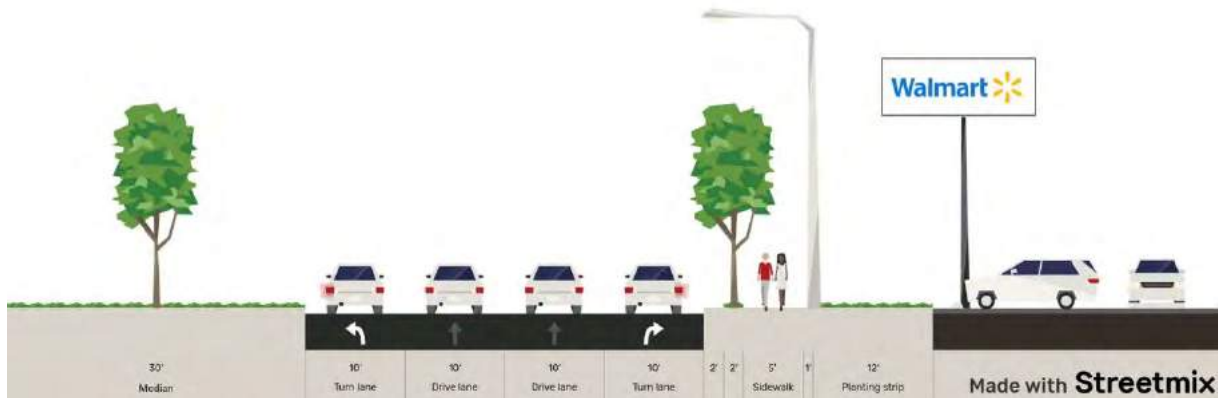
Figure 15: The northbound lane of US13 in front of Walmart, facing northward. This design includes a five-foot sidewalk (a continuation of the existing sidewalk) and planted trees (used to represent various plantings). Created using Streetmix.
