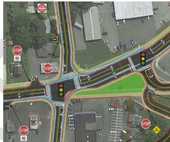
Figure 12: A proposed reconfiguration of the Rehoboth, Walnut, Church, and 10th intersection for improved safety. Source: NW & NE 10th St/N. Church St/ N. Rehoboth Boulevard/ N. Walnut Street Intersection Study (2023) ( link ).
