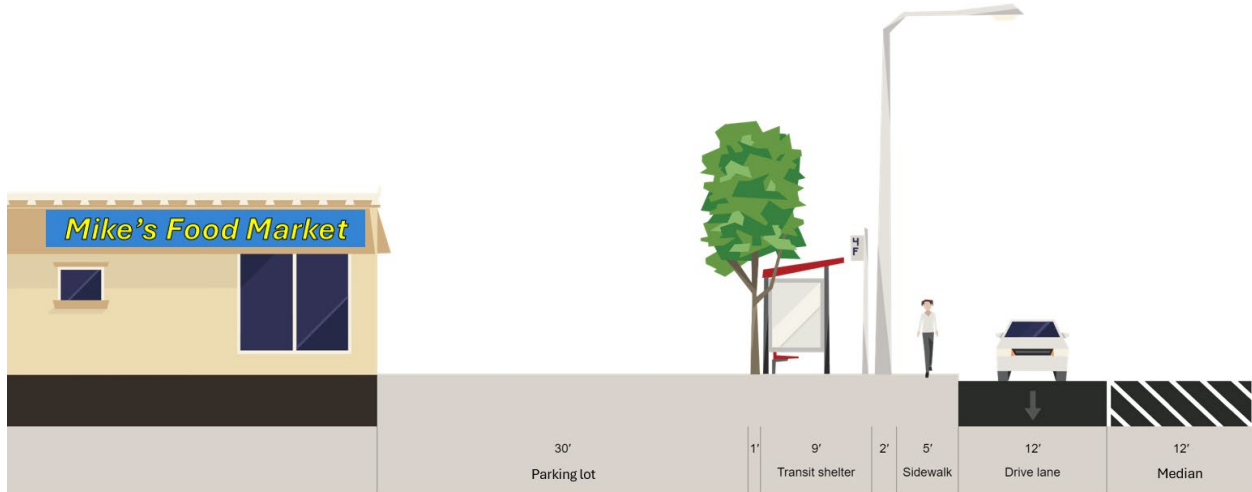
Figure 13: The southbound lane of North Rehoboth Boulevard in front of Perdue, facing northward. This design includes a five-foot sidewalk, a transit shelter, and street lighting. Created using Streetmix.
