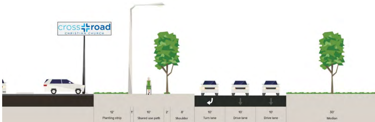
Figure 17: The southbound lane of US13 in front of Walmart, facing northward. This design includes a ten-foot shared use path and planted trees (used to represent various plantings). Created using Streetmix.
