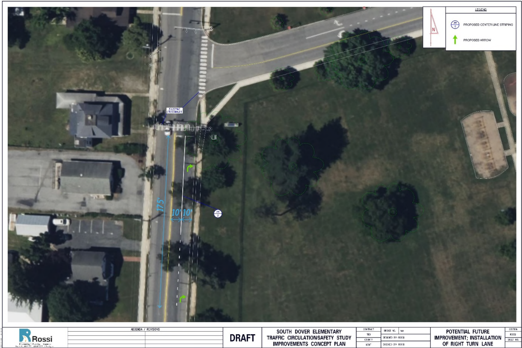
Figure 14: Recommendation B: Installation of Right-Turn Lane at South State Street Intersection
