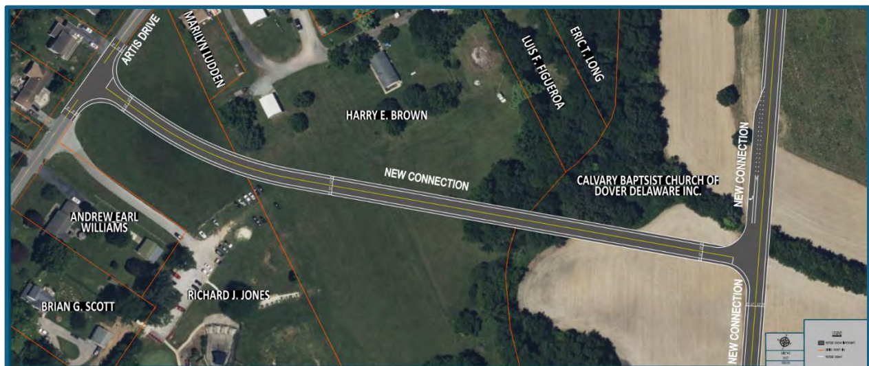
Figure 13 Connection Concept 1 from New Connector to Artis Drive
