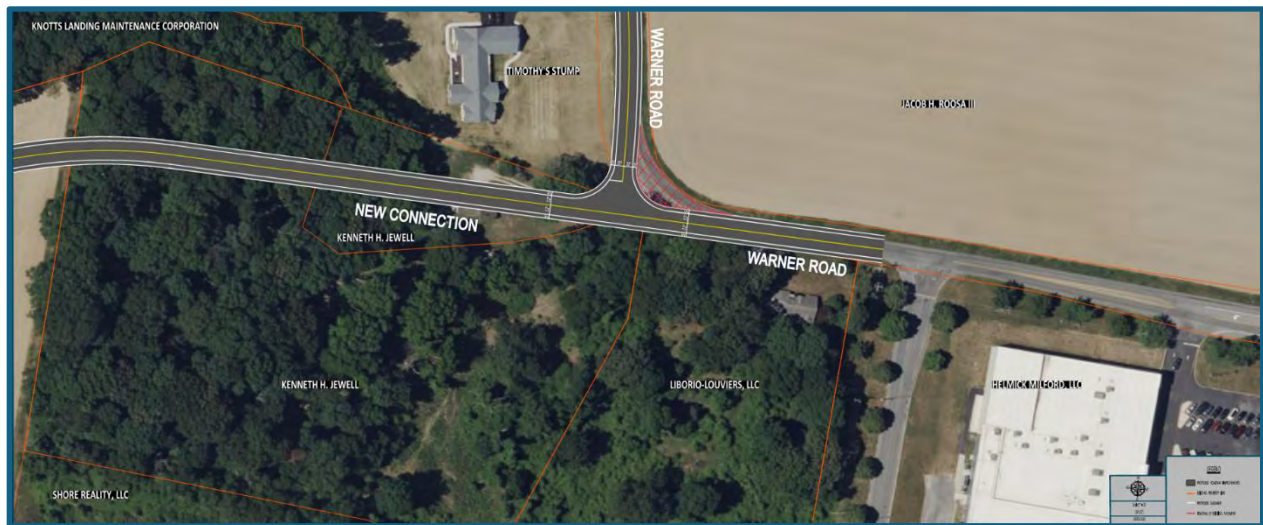
Figure 23 Warner Road Intersection with New Connector
