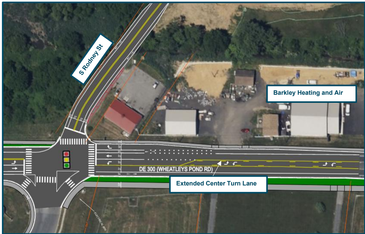
Figure 12 Wheatley's Pond Rd Widening with Extending Center Turn Lane
