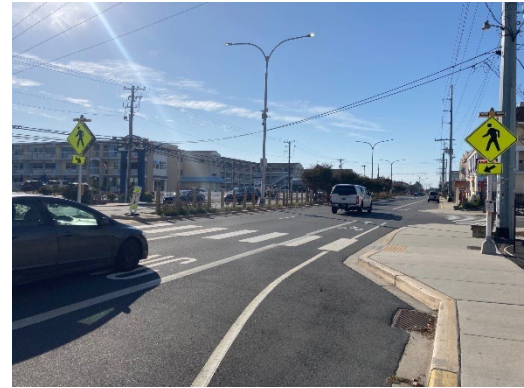
Figure 21: A Rectangular Rapid Flashing Beacon (RRFB), flashing sign, and pedestrian refuge island in Dewey Beach. RRFBs are commonly used in the beach communities of Sussex County.
