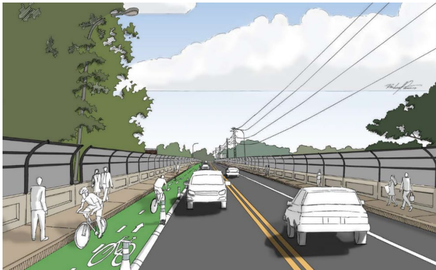
Figure 31. Sketch of cycle track in shoulder on Augustine Cut Off Bridge in Wilmington, Delaware
